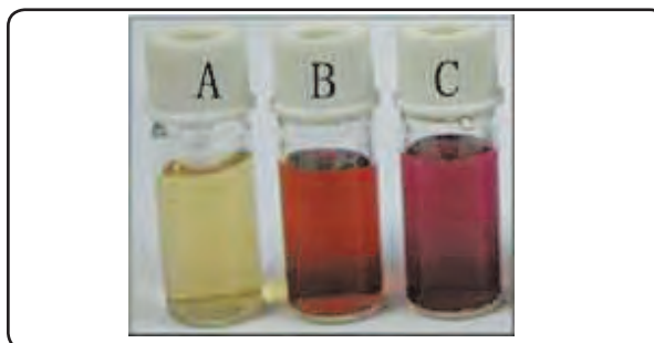
Fig. 16.4 Formation of gold nanoparticles solution
